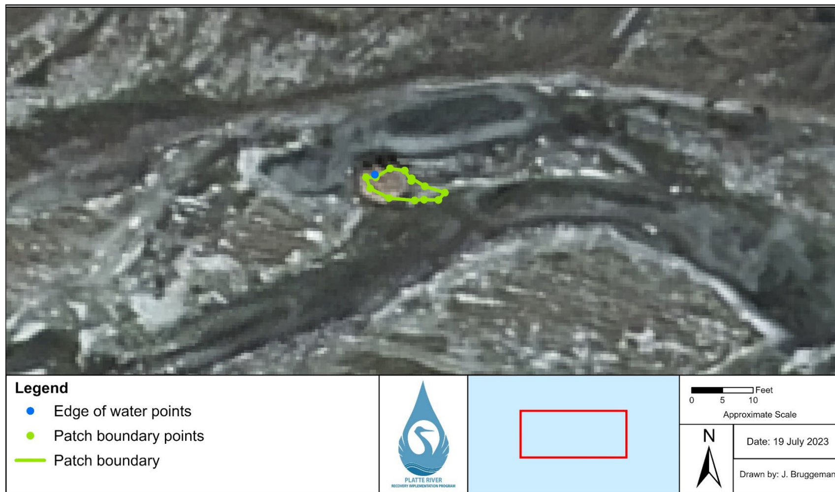
Figure 12. Example of delineated boundaries of a bankline Phragmites patch (green circles and line) surveyed during June 2023 and corresponding water surface elevation measurement (blue circle). Circles depict RTK points. Satellite imagery shown is from fall 2022 and does not depict water conditions during the time of the May 2023 survey.
