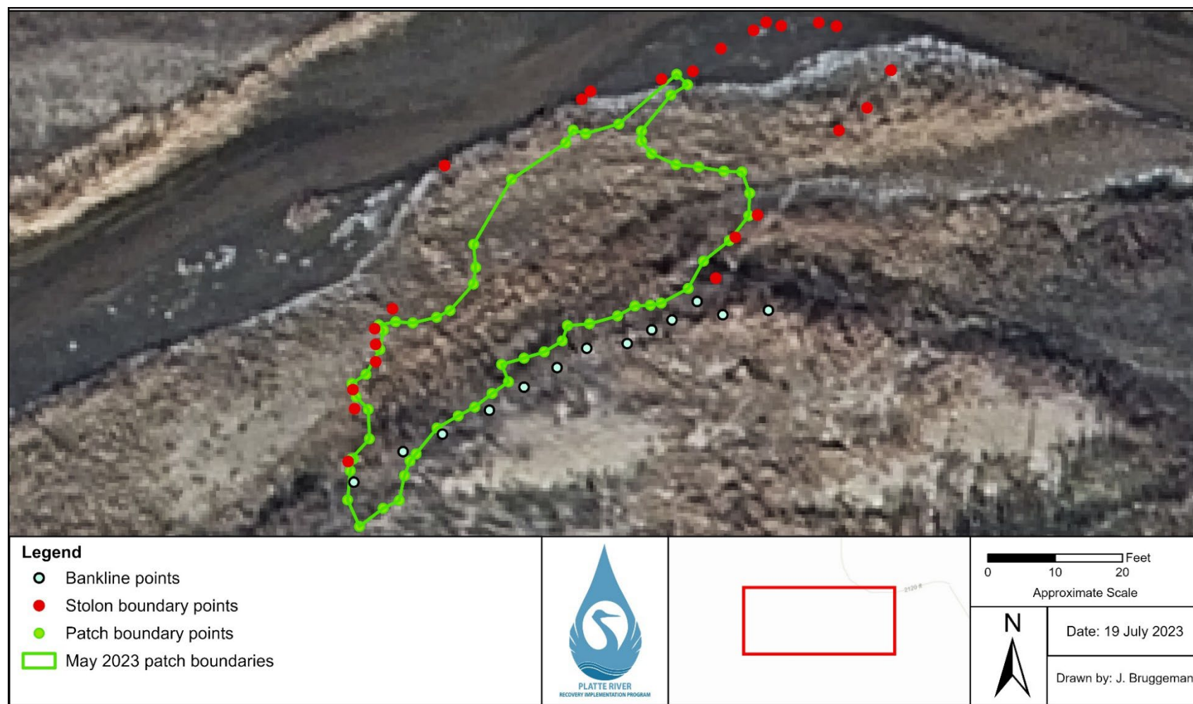
Figure 7. Example of delineated boundaries of a bankline Phragmites patch (green circles and line), stolon reach (red circles), and river channel bankline (light green circles) surveyed during May 2023. Circles depict RTK points taken to define the boundaries. Satellite imagery shown is from fall 2022 and does not depict water conditions during the time of the May survey.
